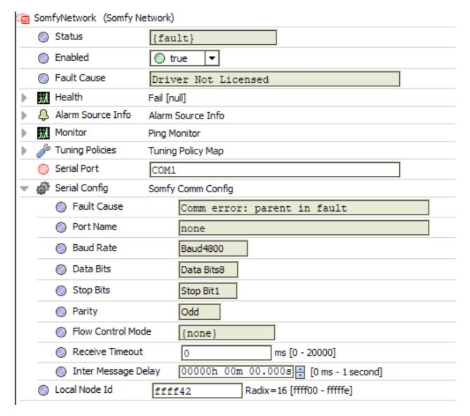
Configure the COM Port to the target RS485 port (e.g. COM1 / RS485-1 etc). The baud rate other communication parameters are fixed and not adjustable.
