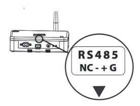
The maximum cable length is 1000m. If a long network is being used it is recommended to terminate the RS485 with 120 Ohm Resistor.
