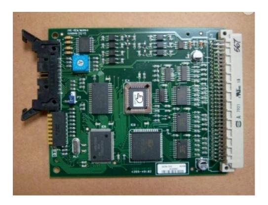
Set the baud rate to 19200 8E1 via rotary switches. Setting No.3 of the rotary switch.
