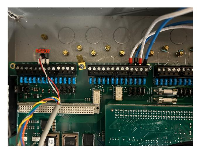
On the panel the communications interface must be configured:
