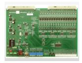
16-way universal input and output cards. Both cards are Modbus RTU enabled with a selectable address and baud rate by way of on-board DIP switches.
